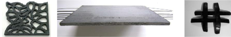
URBAN LIGHT: concrete samples. Note the piece at the top with 0.5 cm thickness.
