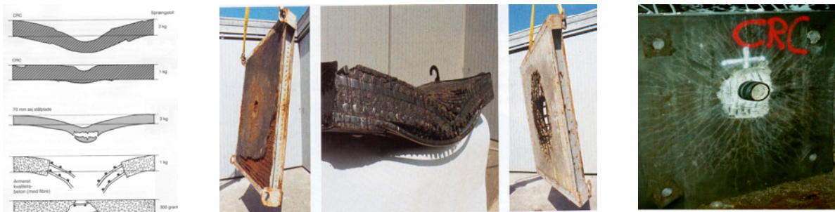
Figure 6. Different kinds of explosive tests and tests where materials are exposed to grenades fired from a canon. The CRC-panels were deformed but not destroyed like both the panels of a strong conventional reinforced concrete and the panels of construction-steel were when exposed to explosives. In the last picture the second panel of CRC catches a grenade of 45 kilo. There were 5 panels of CRC; the three last panels were intact. In comparison it should be mentioned that the grenade continued right through the five panels of strong conventional reinforced concrete and destroyed them completely. (1). (10).
