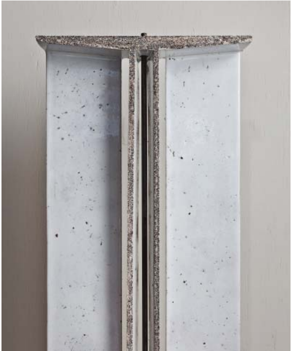
Ceramic Glazed Concrete, selfsupporting facing construction 160-50-1-3 cm. Anja Margrethe Bache, Photos Ole Akhøj.
